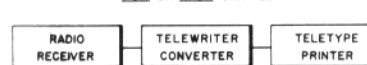
BLOCK DIAGRAM EQUIPMENT NEEDED TO RECEIVE RADIO TELETYPEWRITER FSK OR AFSK SIGNALS
