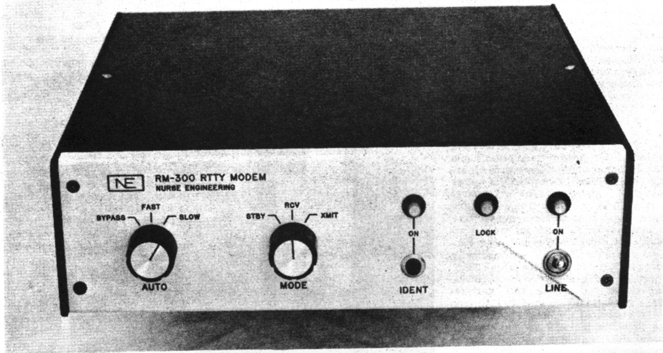
FIGURE 1: Front view of a completed RM-300 Modem. The front panel was engraved at an engraving shop for a cost of $.15 per letter.
