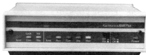
Kantronics KAM Plus with lightning fast G-TOR
